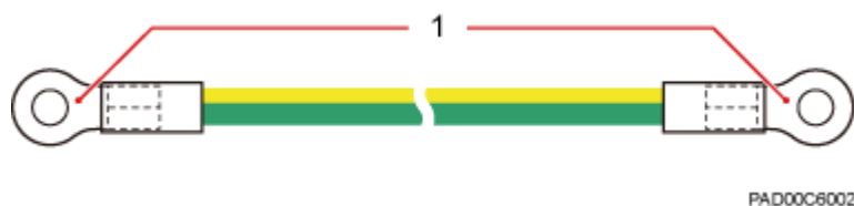
Figure 4-1 Appearance of the PGND cable
