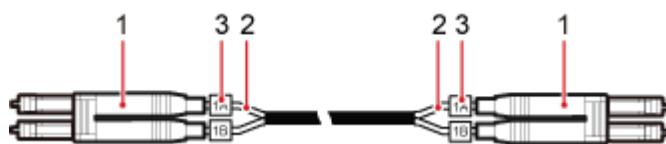
Figure 4-6 FE/GE optical cable (2)
