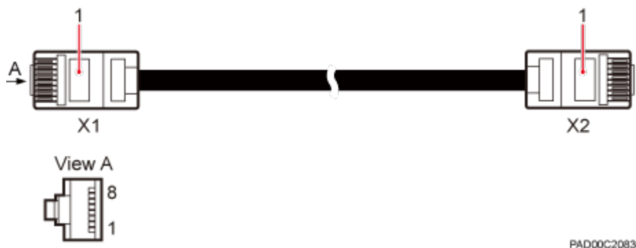
Figure 1-11 Appearance of an Ethernet cable
